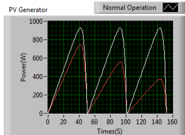
Fig7. Blocking diode reversed polarity influence on the PV generator operation.
