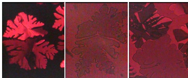
Figure 3. Mesophase domains growing from the isotropic liquid between glass plates on cooling through the liquid to mesophase transition of 16b (left, pseudohomeotropic with residual birefringence), 16c (center, homeotropic) and 4d (right, homeotropic that transits to birefringent during growth: only the bottom domain is still homeotropic). Polarizing optical microscopy (POM) with crossed (left) or slightly uncrossed (center, right) polarizers, 0.24 mm × 0.30 mm.
