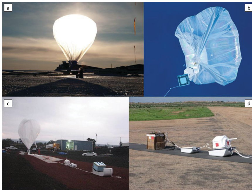
FIG. 5. Four images of driftsonde deployments. (a) Launch from McMurdo Station, Antarctica, during Concordiasi (2010). (b) Shortly after launch during Concordiasi. Dropsondes are visible at the perimeter of the driftsonde gondola below the CNES superpressure balloon. (c) Launch from Hawaii during T-PARC (2008). Driftsonde gondola is on its deployment sled. (d) Driftsonde before launch during AMMA (2006). This earlier version of the driftsonde gondola was constructed from cardboard rather than hard foam.
