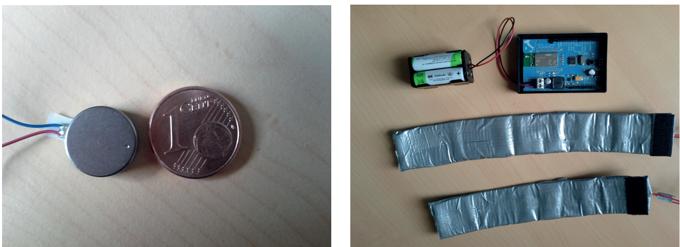
Figure 1: Photograph of the vibrating wristbands. (a) The vibrating motor. (b) The haptic bracelets with Arduino board.
