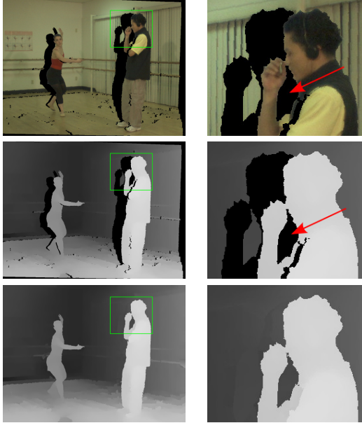
Fig. 1: Illustration of one of the background recovery problems : The hole pointed by the arrow is only surrounded by foreground pixels. Top: synthesized intensity image with holes, middle: synthesized depth map with holes, and bottom: our depth map inpainted result.
