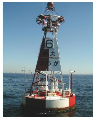
(b) Yoshio Masuda oscillating water column.
