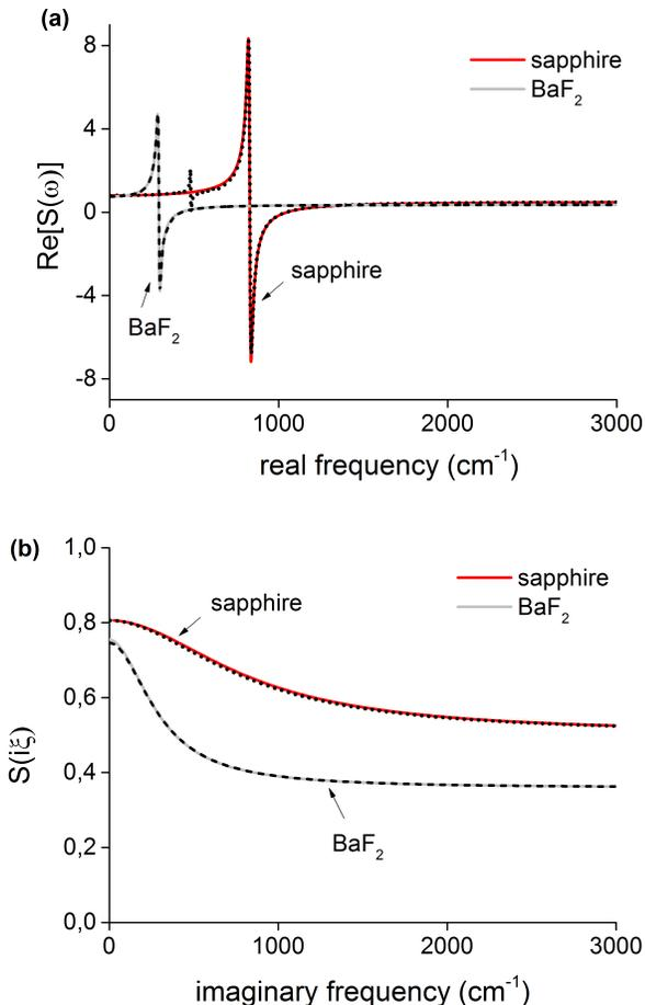
FIG. 1. (Color online)(a) The real part of the surface response for real frequencies. The results of the hydrodynamic model, eqn. (9) are shown for sapphire (red or dark grey) and  $BaF_2$  (grey). The black dotted (sapphire) and dashed ( $BaF_2$ ) lines represent the results of the elaborate model of ref. [36]. (b) The surface response for imaginary frequencies using the exact same colour/line coding. The dielectric constant and therefore the surface response are strictly real in this case.
