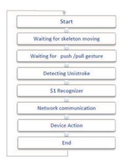
Figure 5: Diagram of gesture recognition using Kinect
