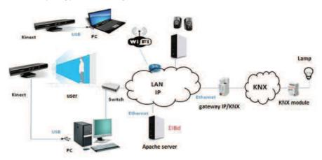
Figure 7: Network Interconnection IP/KNX
