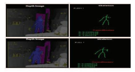
Figure 4: Recognition of push and pull gesture
