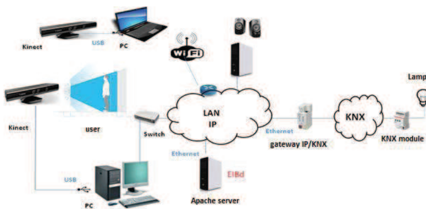
Figure 7: Network Interconnection IP/KNX
