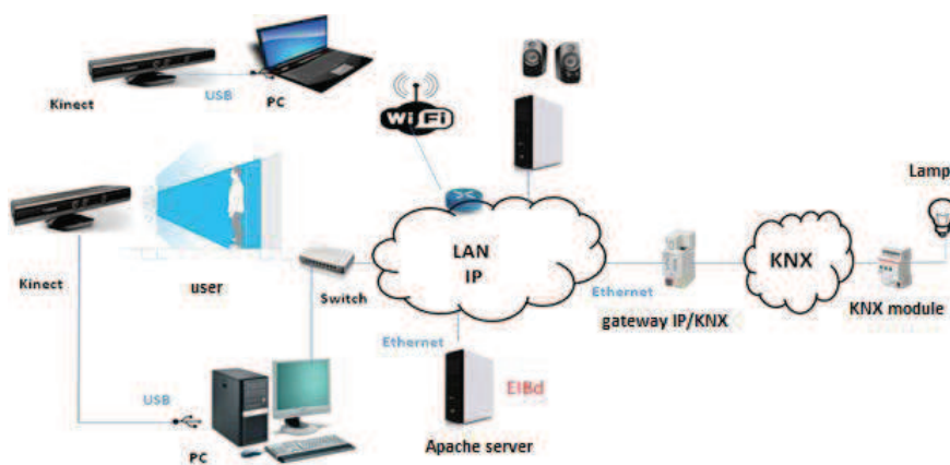
Figure 7: Network Interconnection IP/KNX
