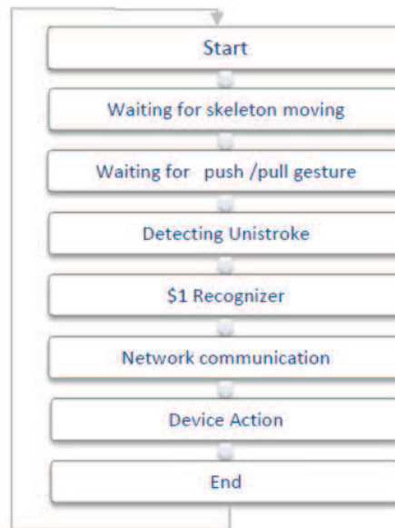
Figure 5: Diagram of gesture recognition using Kinect
