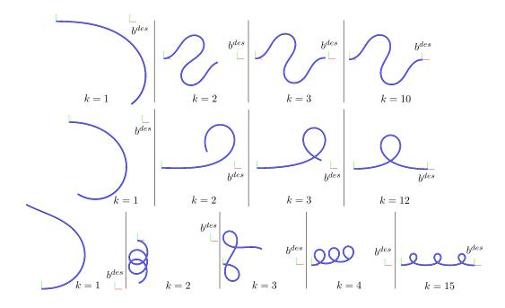
FIGURE 1. Planar rod inverse geometry using Newton's method. The same rod tip position  $b^{des}$  is used with three different initial guesses  $a_0$ , leading to different solutions  $a^*$  corresponding to "wavelike" configuration(top) or "orbit-like" configurations (middle and bottom).
