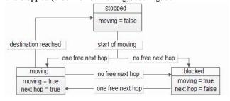
Figure 5. State machine for block motion.
