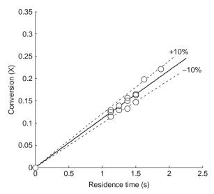
Figure 4 Actinometer conversion versus irradiation time in the microphotoreactor A. Experimental conversions (O) and conversions predicted by eq. (18) (–)
