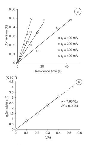
**Figure 5** (a) Actinometer conversion versus irradiation time in the microphotoreactor B for different current intensities supplying the UV-LED array. Experimental conversions (symbols) and conversions predicted by eqs (15)–(17) (straight lines). (b) Photon flux received versus the current intensity supplying to the UV-LED array
