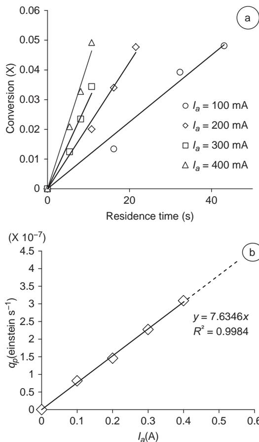
**Figure 5** (a) Actinometer conversion versus irradiation time in the microphotoreactor B for different current intensities supplying the UV-LED array. Experimental conversions (symbols) and conversions predicted by eqs (15)–(17) (straight lines). (b) Photon flux received versus the current intensity supplying to the UV-LED array
