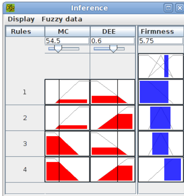
Figure 11: Firmness inference with implicative rules and a precise value
