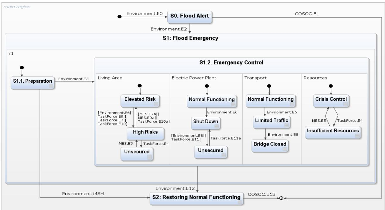
Fig.4. Statecharts diagram of COSOC flood management process
