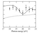
FIG. 2. Experimental and theoretical variation of the asymmetry parameter,  $\beta$ , around the plasmon resonance for HOMO (left) and HOMO-1 (right). Dots: experimental data points. Curves: TDLDA calculation with the inclusion of the plasmon resonance at 20 eV (plain) or without including the plasmon resonance (dashed).
