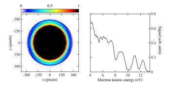
FIG. 1. (Color online) 2D projection of the photoelectron velocity distribution (left) and corresponding angularly integrated photoelectron kinetic energy spectrum (right) for  $C_{60}$  measured at synchrotron photon energy of 20 eV. The two peaks at 12.4 eV and 11.1 eV correspond to ionization from the HOMO and HOMO-1 orbitals, respectively.
