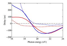
FIG. 3. (Color online) Variation of photoemission time delays for HOMO (red) and HOMO-1 (blue) photoelectrons with photon energy calculated in TDLDA. Corresponding delays without the correlation phase  $\varphi_{\rm C}$  are shown in dashed curves.
