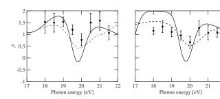
FIG. 4. Comparison between TDLDA and semiclassical calculations of variation of the asymmetry parameter  $\beta$  around the plasmon resonance for HOMO (left) and HOMO-1 (right). Plain curves: semiclassical model calculation. Dashed curves: TDLDA calculation. Dots: experimental data points.
