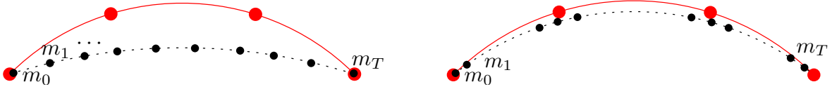
Figure 4: Illustration of Remark 1.6. The set S is the red curve and the set S_N is composed of the four large dots. The discretized geodesics is displayed as a dotted line. On the left, the penalization parameter \lambda is too small and the discretized geodesics takes “shortcuts”, while on the right \lambda is too large, leading to overfitting.
