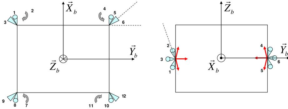
Figure 1: Thruster configuration of the chaser spacecraft<sup>2</sup>
