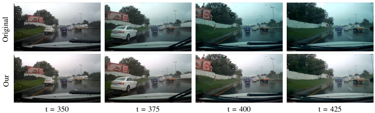
Fig. 4. Tonal stabilization of the sequence “driving”. Top row: frames extracted from the original sequence, t = (350, 375, 400, 425) . Second row: same frames from top row, after tonal stabilization with our method. This video, taken while driving in a highway, is particularly challenging because of the driving speed, the fast motion of objects, the rain droplets falling and the wiper blade movements. Still, our method produces satisfactory tonal stabilization for this sequence, with no artifact creation.
