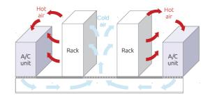
Fig. 1. Architecture of a datacenter with cold/hot aisle.
