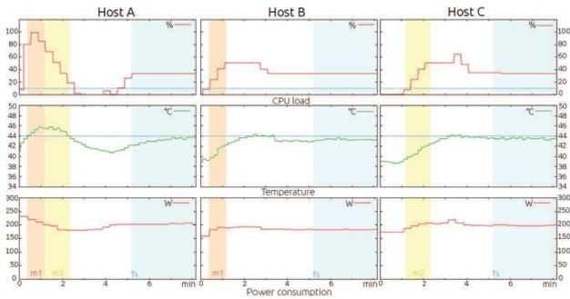
Fig. 6. Stable state reached at time  $T_s$  as the OVERHEAT anomaly threshold is at  $44^{\circ}\text{C}$  compared to  $42^{\circ}\text{C}$  in Fig. 5.  $m_1$  corresponds to migrations from Host A to B and  $m_2$  to migrations from Host A to C
