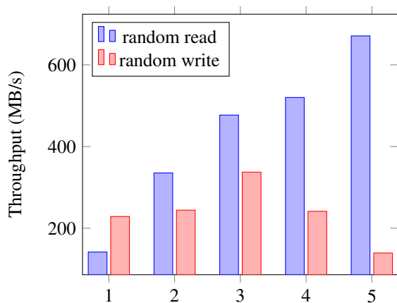
Figure 5: Accumulated throughput (in MB/s) recorded by the threads, depending on the number of clients working in parallel, for random access operations.
