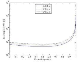
Fig.9 Load capacity versus relative eccentricity with Reynolds conditions
