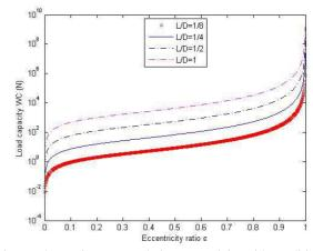
Fig. Load capacity versus relative eccentricity with conditions of short bearing
