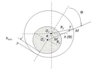
Fig.3. Film thickness between shaft and bearing
