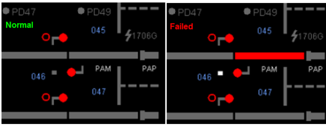
Figure 5: Interval track circuit failure.
