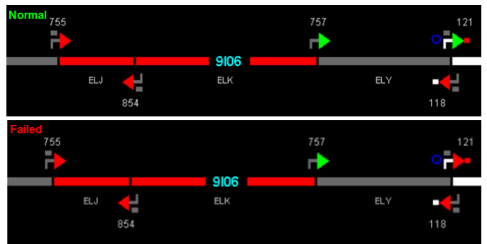
Figure 8: Absolute Stop Marker Route Failure.
