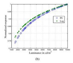
Fig. 2: Comparison of responses for two transformation functions in two different ranges of luminance, (a) 1 - 200 cd/m<sup>2</sup>, (b) 1000 - 10000 cd/m<sup>2</sup>. Figure best viewed in color.
