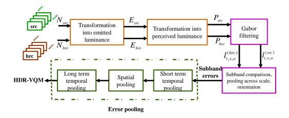
Fig. 1: Block diagram of the proposed HDR-VQM.
