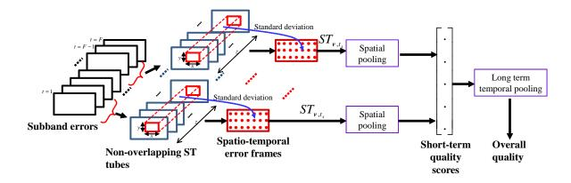
Fig. 3: Error pooling in HDR-VQM.
