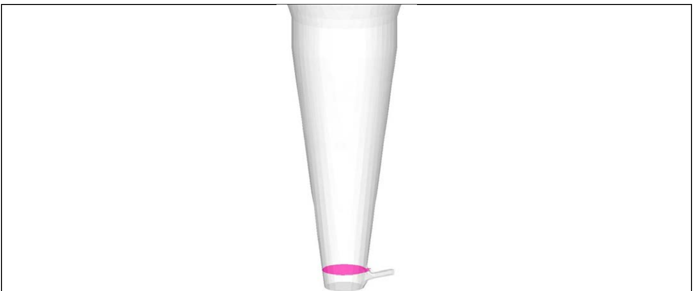
Figure 8 : Virtual plane above the air injection to evaluate the solid circulation
