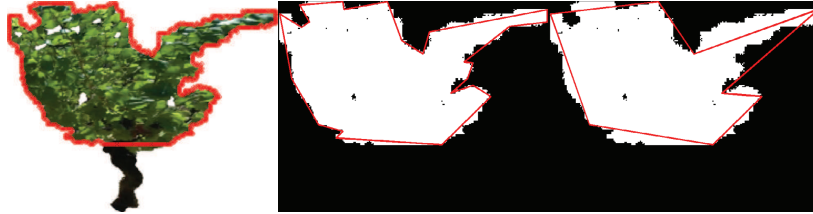
Fig. 5. DCE algorithm examples. At the left, the original image with the contour points around the foliage. The two other images show the DCE algorithm with a 24-point polygon in the middle and a 8-point polygon on the right. The inward angles are represented in blue.
