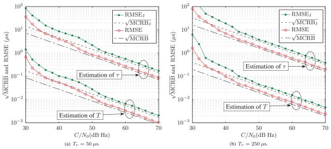
Fig. 4. Performances for TOA and symbol width estimation for (a) minimum and (b) maximum rise times allowed on the SAR system.
