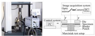
Fig. 2. Marciniak test setup and its schematic illustration.
