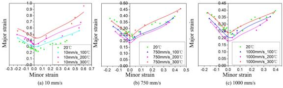
Fig. 6. Comparison of forming limit curves for different temperatures at given punch speed.
