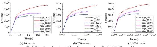
Fig. 1. Comparison of experimental force-time curves and ones fitted with Lin-Voce model.
