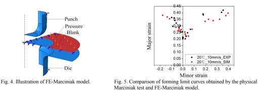
Fig. 5 shows the forming limit curves obtained by the physical Marciniak test and FE-Marciniak model at the punch speed of 10 mm/s at room temperature. A great consistency can be observed, which also proves that Lin-Voce constitutive model is suitable for describing the deformation behaviour of AA5086 under different strain conditions.
