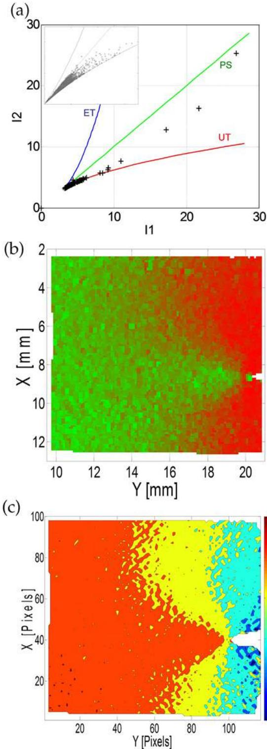
**Fig. 4.** Heterogeneity of stretch states at the end of the loading phase. a) Distribution in the  $(I_1, I_2)$  plane. b) Distribution over the ROI. Colors range from red for UT to green for PS. c) Map of biaxiality ratios  $b$ . (For interpretation of the references to color in this figure legend, the reader is referred to the web version of this article.)
