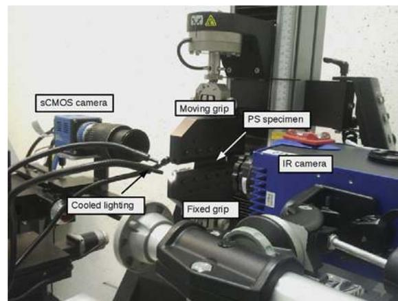
**Fig. 2.** Experimental device.
