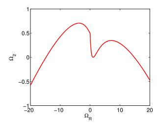
Figure 3: Angular rate associated with the mean zonal flow generated by an elliptical forcing, n = 2 in the cylinder (solid red line) as a function of  $\Omega_R$ .
