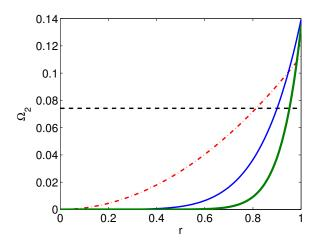
Figure 4: Angular rate associated with the mean zonal flow generated by various multipolar forcings in the cylinder for  $\Omega_R = 2$ . The dashed black line is an elliptical forcing, n = 2; the dashed-dotted red line is a tripolar forcing, n = 3; solid blue line corresponds to n = 5, and the solid thick green line is n = 8.
