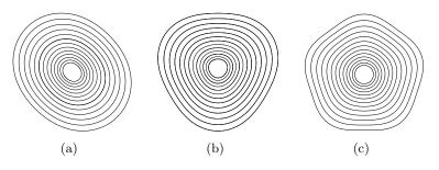
Figure 2: Streamlines induced by multipolar deformation with  $\beta = 0.1$  and  $r_{moy}$  ranging between 0.45 and 1 for (a) n = 2, (b) n = 3 and (c) n = 5.
