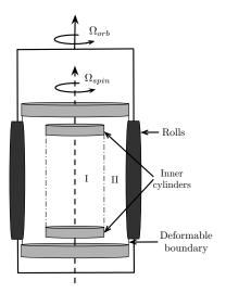
Figure 1: Experimental setup corresponding to the situation described in this paper for n = 2. A flexible outer cylinder rotating at an angular velocity  $\Omega_{spin}$  is deformed by two rolls rotating at a constant angular velocity  $\Omega_{orb}$ . It generates elliptical streamlines in the bulk. Two cylindrical plates rotate at the velocity of the outer cylinder,  $\Omega_{spin}$ . We are interested by the zonal flow generated in region I.
