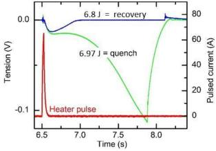
Fig. 2. Illustration of MQE at  $T=10~K,\,B=8~T,\,Icoil=280~A.$  The heater pulse (red) initiates a disturbance which recovers (blue) or grows to a quench (red).
