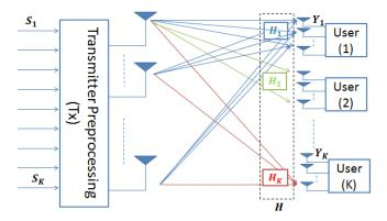
Fig. 1. Diagram of MU-MIMO system.
