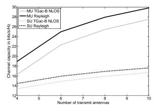
Fig. 5. Capacity value achieved by an i.i.d Rayleigh and TGac-B NLOS channels.
