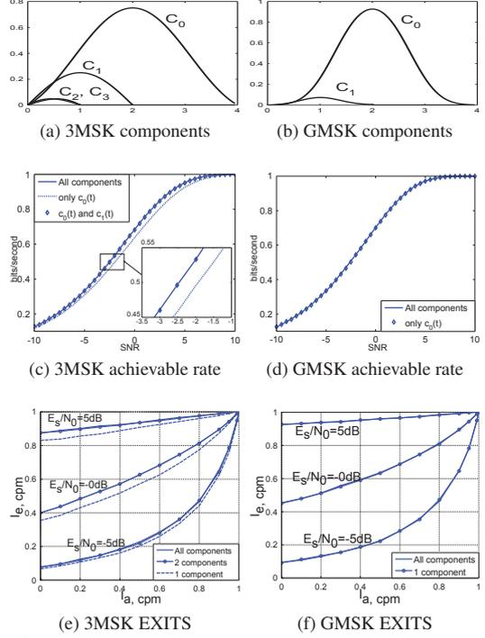
Fig. 2: Laurent components,  $R^*$  rate and EXIT for GMSK and 3MSK
