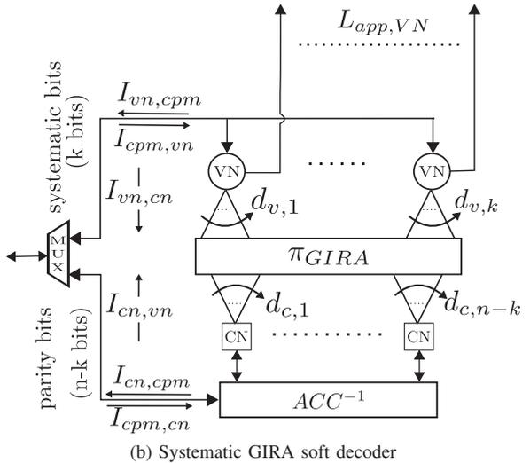
Fig. 1: GIRA encoder and decoder
