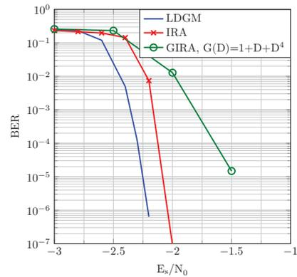
Fig. 7: Obtained BER of GIRA codes with GMSK
