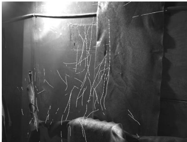
Fig.10. PTV measurement over a heater in a room [16]
