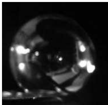
Fig. 3. Single helium filled soap bubble. Light scattered on the shell can be seen. [45]
