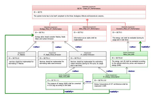
Figure 4. System requirements SysML Diagram
