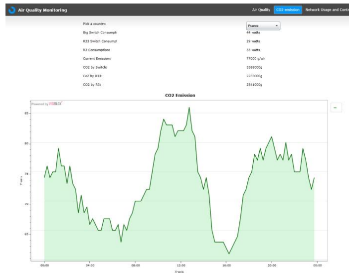
Figure 6. Monitoring ICT Energy consumption and Carbon emission
