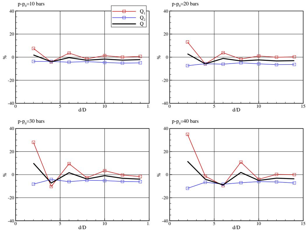
**Figure 7:** Perturbations of the energy absorption by wave interactions in an array of two systems as a function of their distance, in regular waves.
