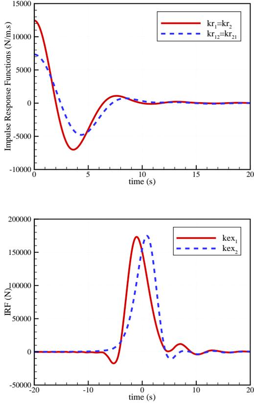
**Figure 2:** Impulse Response Functions (IRFs) of the radiation and excitation forces in heave in the case of two cylinders separated by a distance of 20 m. One could notice that the amplitude of the crossed IRF  $k_{12}$  of the radiation force is the same order as  $k_1$ .
