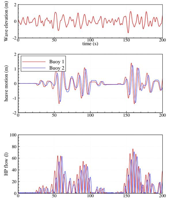
**Figure 3:** Time series of the free surface elevation (top), of the heave motion (middle) and of HP flow (bottom) of two generic wave energy converters. Characteristics of the monodirectional incident wave are  $T_p = 10$  s,  $H_s = 2$  m and  $\gamma = 3.3$ . The distance between the two cylinders is 20 m.
