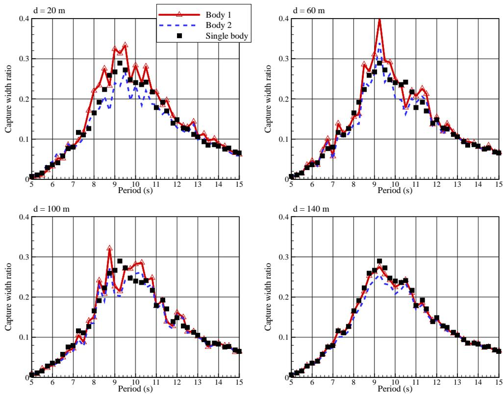
**Figure 9:** Capture width ratios of the first buoy and of the second buoy as a function of distance between them in irregular seas. In these simulations,  $\Delta p = 10$  bars and the wave amplitude was set equal to 2 m.
