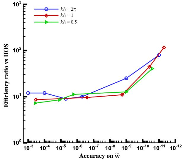
Figure 11. Influence of  $kh$  on efficiency ratio between *OceanWave3D* and HOS.
