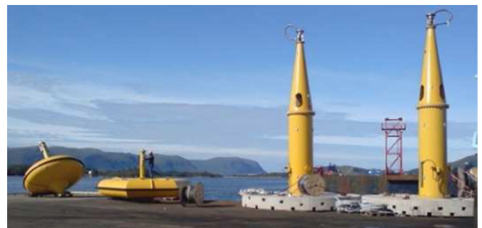
Fig. 1. Components of the Seabased WEC.
