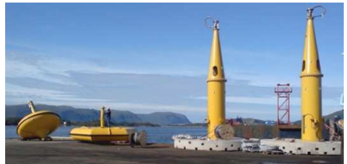
Fig. 1. Components of the Seabased WEC.
