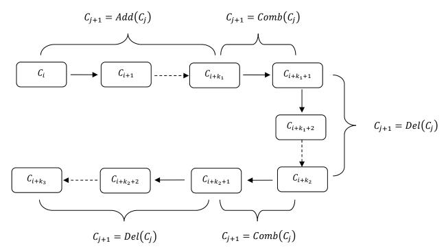
Fig. 3 Diagram of operations scheduling during a branch reconfiguration in a stage with BpBAR
