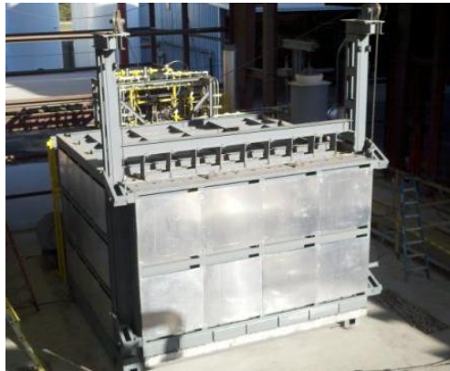
Figure 2. Example of a forge furnace
