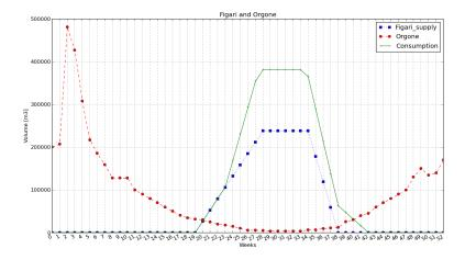
Fig. 15. The optimal solution for the Figari dam.
