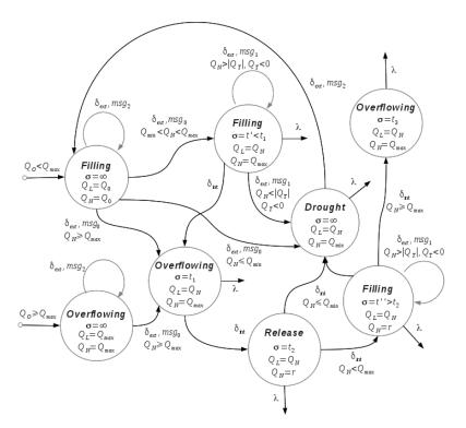
Fig. 8. The state graph of the DAM model.
