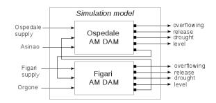
Fig. 9. DEVS simulation coupled model of the catchment basin.
