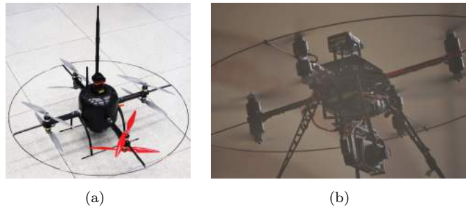
Figure 21. Standard NIFTi UAV octocopter with a standard configuration (a) and NIFTi UAV research octocopter (b) with a mounted on top camera, and a camera in a tilt unit under the main body. Another configuration flow includes a PC and a Kinect-style sensor mounted on top of the research UAV.
