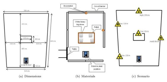
Figure 19. Set-up of the detect objects task
