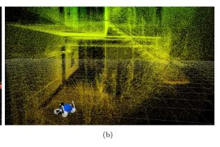
Figure 4. (a) Assembled point cloud with color information. (b) 3D Point cloud map of a staircase.
