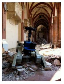
Figure 20. NIFTi UGV with a rotating SICK-Laser (LMS100), a LadyBug3 omnicam, active flippers and active/passive bogeys, IMU, GPS, and a static mast mounting a PTU with a Kinect sensor.
