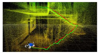
Figure 10. Autonomous descend of a complex staircase. Green line: the initial path planned by the robot. Red line: the actual robot path.
