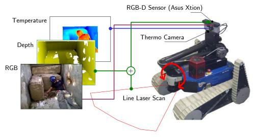
Figure 5. The scheme of multiple modalities (Color, depth, temperature) represented as a layered array computed from different sensors. The Lidar swivels from side to side, capturing full 3D.
