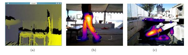
Figure 6. (a) Semi-dense depth computed from laser line scans, while robot undergoes motion (in this case rotation). (b),(c) Examples of human detection. In (c) the false detections are caused by concrete blocks being heated by the sun to the temperature around 36 degrees.
