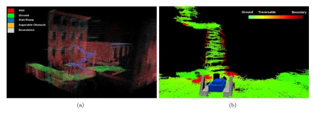
Figure 12. (a) Point cloud segmentation and labeling and (b) weighted graph representation of a fire escape stairs scenario.
