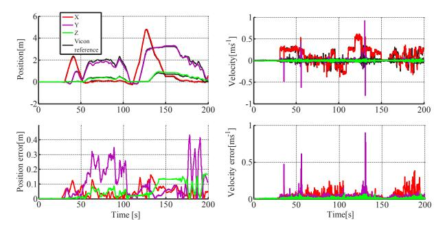
Figure 9: The corrected position (top left) and velocity estimates (top right) for the IMU+OD+ICP+VO combination corresponding to the trajectory in Figure 8 (testing obstacle traversability). Errors in position and velocity are obtained as norm of difference between the Vicon reference and the corresponding state at each time-step (bottom left, bottom right). The Vicon reference for both position and velocity is shown in black.
