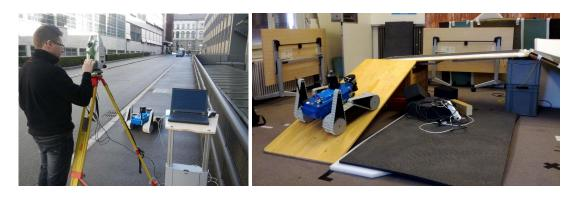
Figure 5: The experimental setup with the Leica reference theodolite for obtaining ground truth trajectory (left). Part of the 3D semi-structured environment for indoor test with motion capture ground truth (right).
