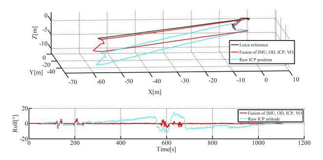
Figure 22: Trajectory estimates in case of map deformation. Solid black line: ground truth; solid red line: state estimate with all four modalities; cyan line: position estimated by ICP alone. Top: side view; bottom: roll angle along the trajectory.
