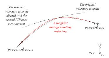
Figure 4: The principle of trajectory approach: when the new ICP measurement arrives (time-step i), trajectory estimate based on measurements other than ICP (black dotted line) is duplicated and aligned with the incoming ICP measurement (black dashed line) and weighted average (red solid line) of these two trajectories is computed.
