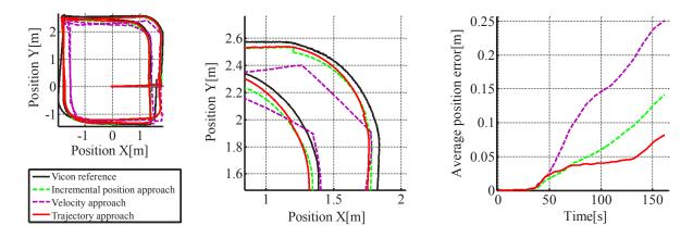
Figure 15: Comparison of effects of the three different ICP aiding approaches on the estimated trajectory (left, middle) and on the average position error (right). Note the *corner cutting* effect of the *velocity approach*.
