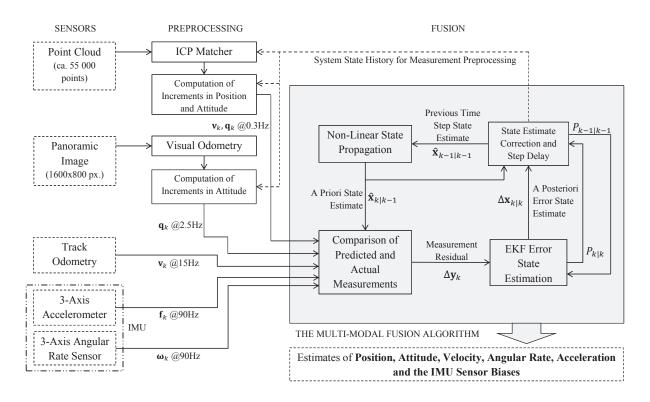
Figure 2: The scheme of the proposed multi-modal data fusion system ( $\omega$  is angular velocity,  $\mathbf{f}$  is specific force (Savage, 1998),  $\mathbf{v}$  is velocity and  $\mathbf{q}$  is quaternion representing attitude).
