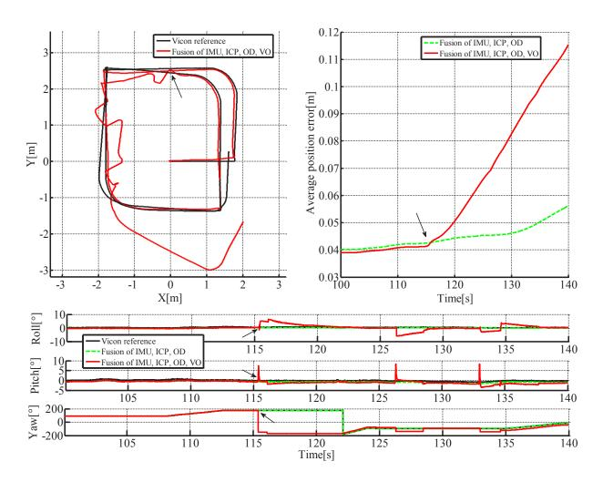
Figure 18: Trajectory reconstruction with partial omnicamera occlusion. Black line: ground truth; Solid red line: state estimate with all four modalities; Dashed green line: state estimate excluding visual odometry; Black arrow: visual odometry failure. Top left: top view of the trajectory; Top right: average position error around visual odometry failure; Bottom: attitude estimated along the trajectory.
