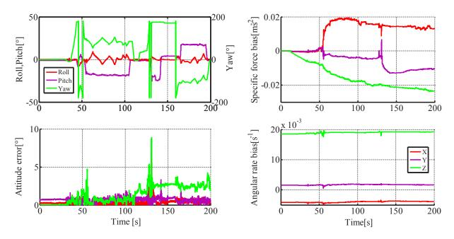
Figure 10: The corrected attitude estimates (top left) for the full multi-modal combination IMU+OD+ICP+VO corresponding to the trajectory shown in Figure 8 (testing obstacle traversability). Errors in attitude are obtained as the difference between the Vicon reference and the corresponding state at each time-step (bottom left). Estimated biases for the specific forces (top right) and angular rates (bottom right).
