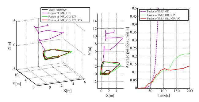
Figure 8: Trajectories obtained by fusing different combinations of modalities during the indoor experiment testing obstacle (depicted in Figure 7) traversability under high slippage (left, middle); development of the average position error (right).
