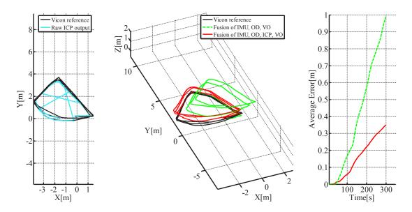
Figure 19: Trajectory estimates in case of low ICP frequency. Black line: ground truth; cyan line: positions estimated by ICP alone; red line: state estimate with all four modalities; green dashed line: state estimate excluding ICP measurements. Left: top view; middle: 3D view; right: average position error.
