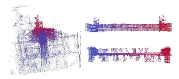
Figure 21: Deformed point cloud map created by ICP. The points are colored alongside the corridor from red (initial position) to blue. Left: front view; top right: side view; bottom right: top view.
