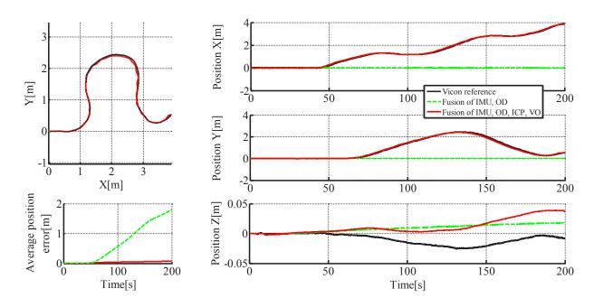
Figure 16: Test trajectory for robot slippage. Black line: ground-truth; red solid line: state estimate with all four modalities; green dashed line: IMU and odometry fusion. Top left: top view of the trajectory; bottom left: average error as a function of time; top, middle, bottom right: evolution of x, y, z coordinate.
