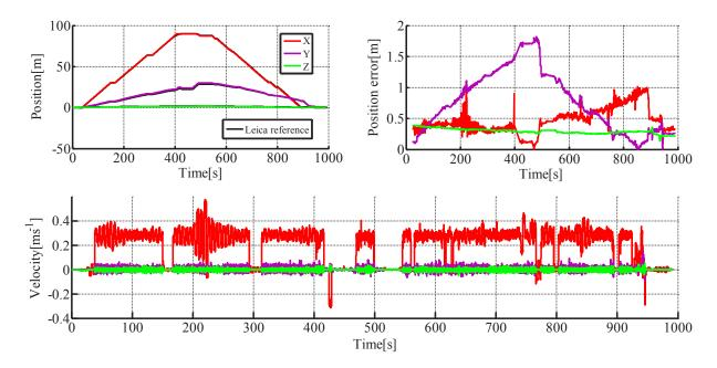
Figure 13: The position and velocity estimates (top left and bottom respectively) for the IMU+OD+ICP+VO combination corresponding to the outdoor trajectory in Figure 12; errors in position obtained as norm of differences between the Leica reference and the corresponding state at each time-step (top right).
