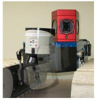
Figure 1: Picture of two USAR UGVs used for experimental evaluation (FP7-ICT-247870 NIFTi project) and a detail of the sensor setup (a PointGrey Ladybug 3 omnicamera and a rotating SICK LMS-151 laser range finder). See Section 3.1 for more details.
