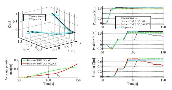
Figure 20: Trajectory estimates in case of moving obstacle in reduced field of view. Solid black line: ground truth; solid red line: state estimate with all four modalities; dashed green line: state estimate excluding ICP measurements; cyan line: position estimated by ICP alone; black arrow: start of moving obstacle. Top left: 3D view; bottom left: average error as a function of time; right: x, y, and z coordinates as a function of time.
