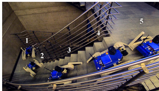
Fig. 1. NiftiBot during autonomous climbing of a curved staircase.
