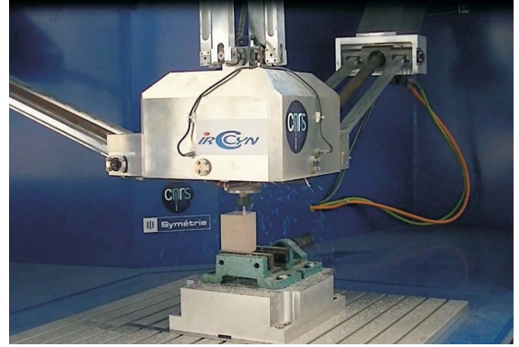
FIGURE 2. Semi industrial prototype of the Orthoglide 5-Axis performing a machining operation
